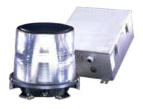
The FT 736 provides highly conspicuous heliport acquisition by flashing an omnidirectional white Morse code "H" (four flashes spaced 2/15 of a second apart at two-second intervals). This flashing pattern readily distinguishes this beacon from other lighting in the area.
